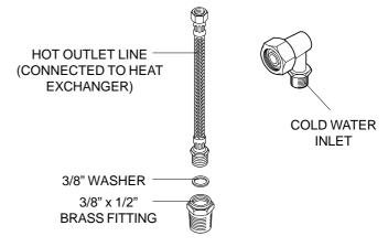
Fig. 3 - Water connections
